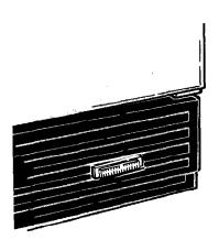
Exterior signal light – Located on the right side of the base grille, automatically indicates any power interruption to the freezer. When power is being supplied. the light will glow If light **does not** glow, check immediately. The electric current may be off; the freezer may be disconnected from the outlet; or the warning light may be burned out.
